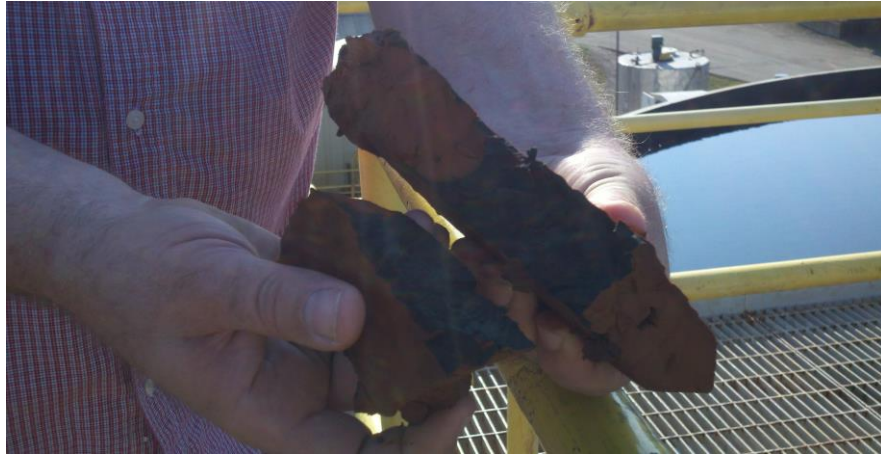
Figure 13: Firm dewatered sludge formed with combined magnesium hydroxide and lime.
