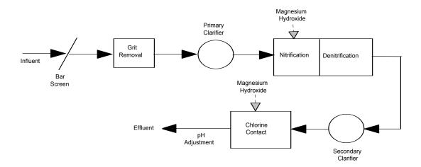
discharge limit. Since magnesium hydroxide is non-toxic and non-corrosive, handling was safer and easier which made magnesium hydroxide the more attractive alkali. Currently, this municipality uses one ton per year (dry solids basis) of MagneClear<sup>TM</sup>58 in their biological treatment system for nitrification and pH adjustment.
